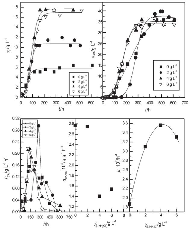
Fig. 6 – Variations in dry biomass, citric acid concentration and productivity with time at different initial ammonium chloride concentrations ( $\gamma_{S,NH_4Cl_0}$ ) and changes in maximum specific citric acid production rate and specific growth rate with  $\gamma_{S,NH_4Cl_0}$  for *Y. lipolytica* 57 ( $\gamma_{S,Go} = 100 \text{ g L}^{-1}$ , initial pH 5.2,  $\vartheta = 30 \text{ }^\circ\text{C}$ )
