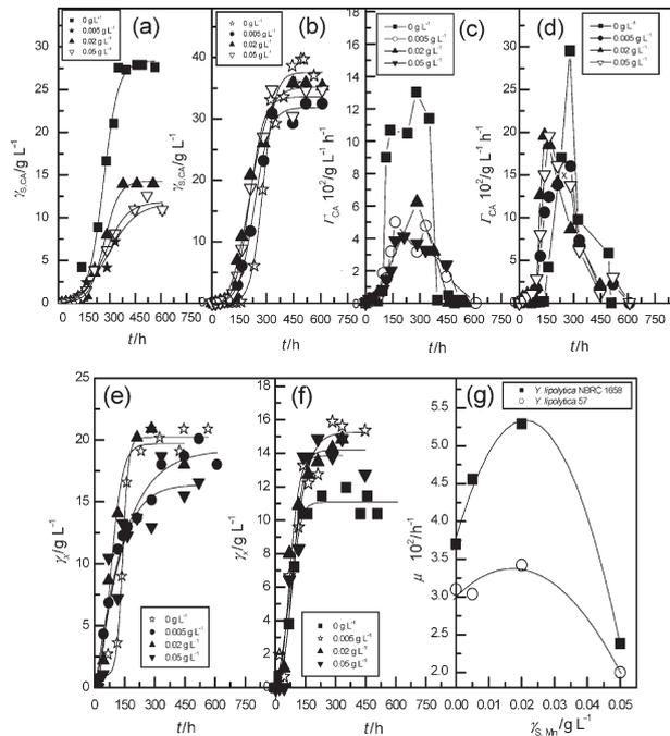
Fig. 7 – Variations in citric acid concentration, productivity and dry biomass with time at different initial  $MnSO_4 \cdot 4H_2O$  concentrations ( $\gamma_{S,Mn}$ ) and changes in specific growth rate with  $\gamma_{S,Mn}$  for the yeast strains (a, c, e, g: *Y. lipolytica* NBRC 1658, b, d, f, g: *Y. lipolytica* 57,  $\gamma_{S,Go} = 100\ g\ L^{-1}$ , initial pH 5.2,  $\vartheta = 30\ ^\circ C$ ,  $\gamma_{S,NH_4Cl,0} = 2\ g\ L^{-1}$ )
