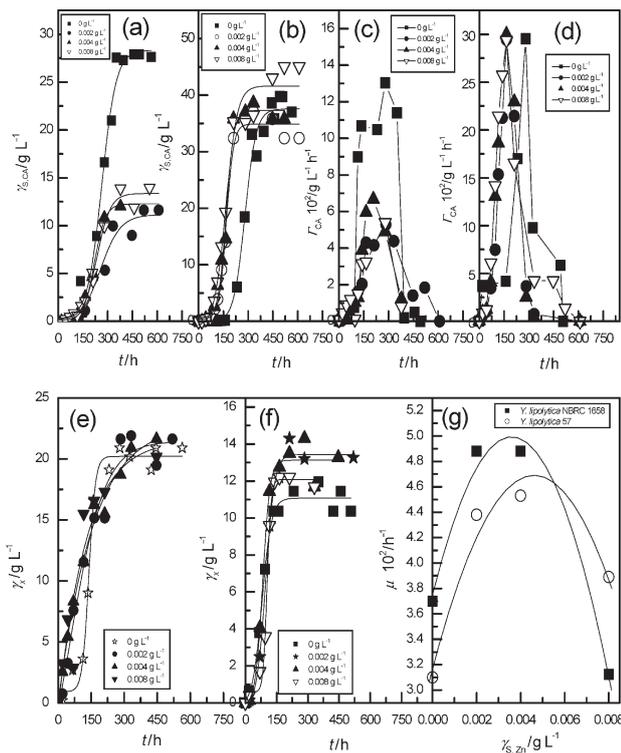
Fig. 8 – Variations in citric acid concentration, productivity and dry biomass with time at different initial  $\text{ZnSO}_4 \cdot 7\text{H}_2\text{O}$  concentrations ( $\gamma_{S,Zn}$ ) and changes in specific growth rate with  $\gamma_{S,Zn}$  for the yeast strains (a, c, e, g: *Y. lipolytica* NBRC 1658, b, d, f, g: *Y. lipolytica* 57,  $\gamma_{S,G0} = 100 \text{ g L}^{-1}$ , initial pH 5.2,  $\theta = 30 \text{ }^\circ\text{C}$ ,  $\gamma_{S,NH_4Cl,0} = 2 \text{ g L}^{-1}$ )
