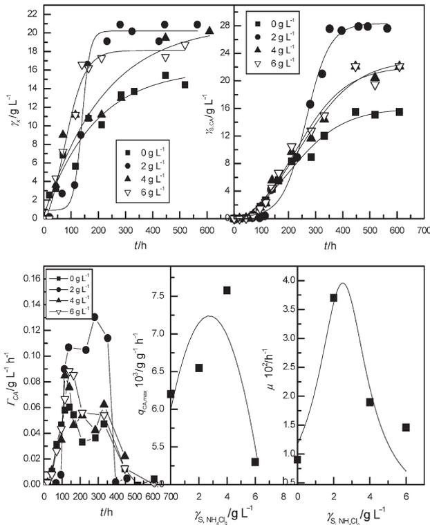
Fig. 5 – Variations in dry biomass, citric acid concentration and productivity with time at different initial ammonium chloride concentrations ( $\gamma_{S,NH_4Cl_0}$ ) and changes in maximum specific citric acid production rate and specific growth rate with  $\gamma_{S,NH_4Cl_0}$  for *Y. lipolytica* NBRC 1658 ( $\gamma_{S,Go} = 100 \text{ g L}^{-1}$ , initial pH 5.2,  $\vartheta = 30 \text{ }^\circ\text{C}$ )
