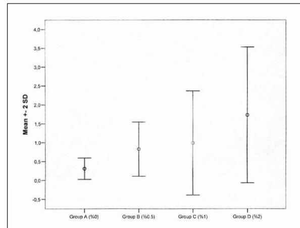
Figure 2. Mean surface roughness values for autopolymerizing resin after reinforced glass fiber with different concentrations.
