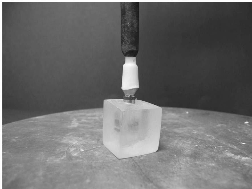
**Fig. 2.** Representative sample of zirconia coping being seated onto the abutments under compression load (20 N) for 10 minutes.
