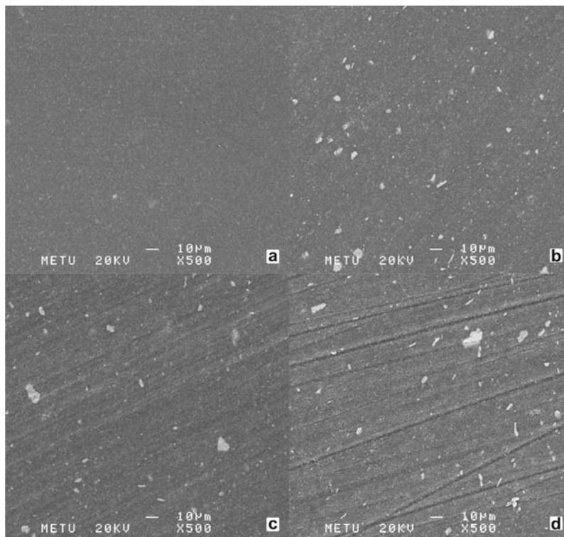
Fig. 4 Compoglass Flow surfaces polished with different systems ( $\times 500$  magnification). (a) Control surface with Mylar strip; (b) Polished with PoGo; (c) Polished with OprtaPol; (d) Polished with Sof-Lex.
