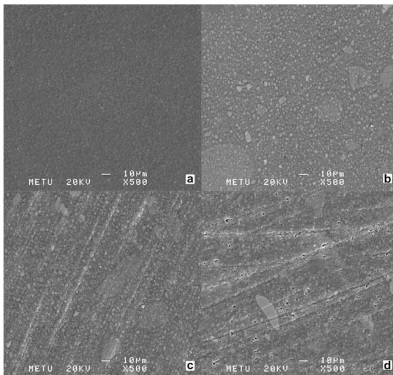
Fig. 5 Filtek Supreme XT Flow surfaces polished with different systems ( $\times 500$  magnification). (a) Control surface with Mylar strip; (b) Polished with PoGo; (c) Polished with OprtaPol; (d) Polished with Sof-Lex.
