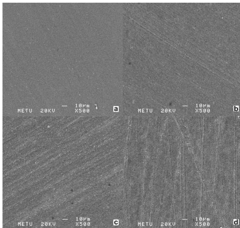
Fig. 3 Admira Flow surfaces polished with different systems ( $\times 500$  magnification). (a) Control surface with Mylar strip; (b) Polished with PoGo; (c) Polished with OprtaPol; (d) Polished with Sof-Lex.
