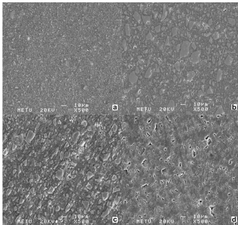
Fig. 2 Grandio Flow surfaces polished with different systems ( $\times 500$  magnification). (a) Control surface with Mylar strip; (b) Polished with PoGo; (c) Polished with OprtaPol; (d) Polished with Sof-Lex.
