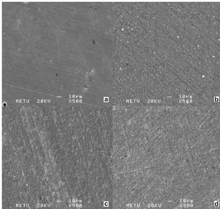
Fig. 6 Filtek Z250 surfaces polished with different systems ( $\times 500$  magnification). (a) Control surface with Mylar strip; (b) Polished with PoGo; (c) Polished with OptrPol; (d) Polished with Sof-Lex.
