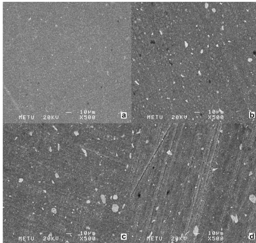
Fig. 1 Tetric Flow surfaces polished with different systems ( $\times 500$  magnification). (a) Control surface with Mylar strip; (b) Polished with PoGo; (c) Polished with OptraPol; (d) Polished with Sof-Lex.
